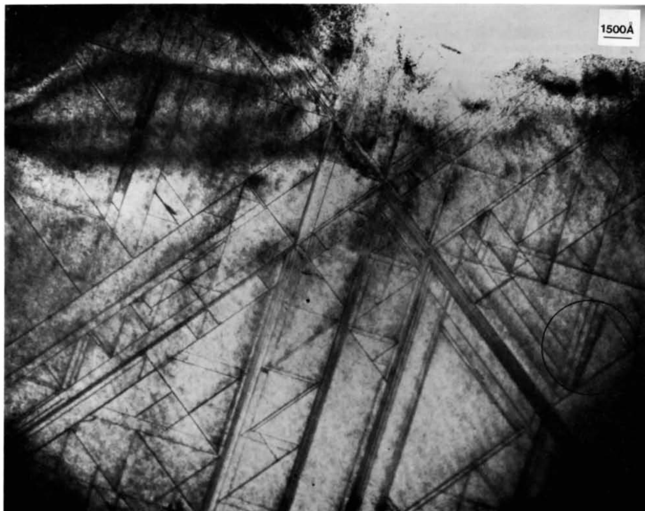
Fig. 9. Low-magnification image showing intersections in ion-thinned Ga-doped rutile. Note the absence of terminations ( cf. T in Fig. 5) and the presence of some lamellae (broad dark bands). Altogether 350 intersections were identified and classified using Fig. 4 (see Table 2).
